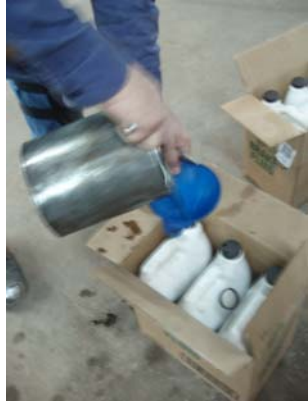
Dispensing of excess brake fluid
