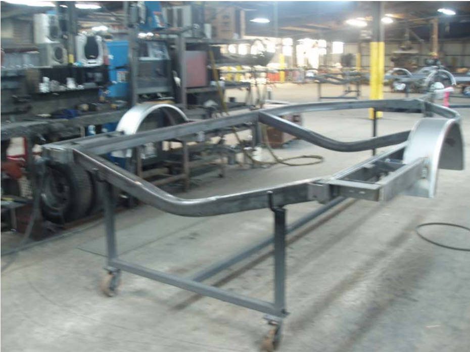
Welded trailer frames are moved through the plant on carts
