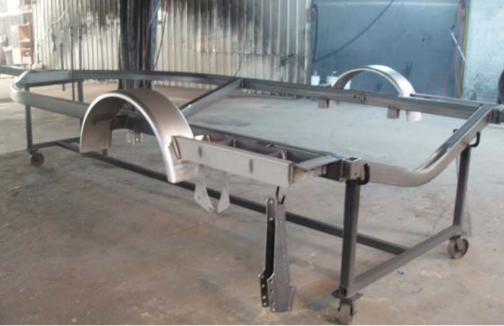
After wash, trailers are dried with air and moved on carts to the paint booth
