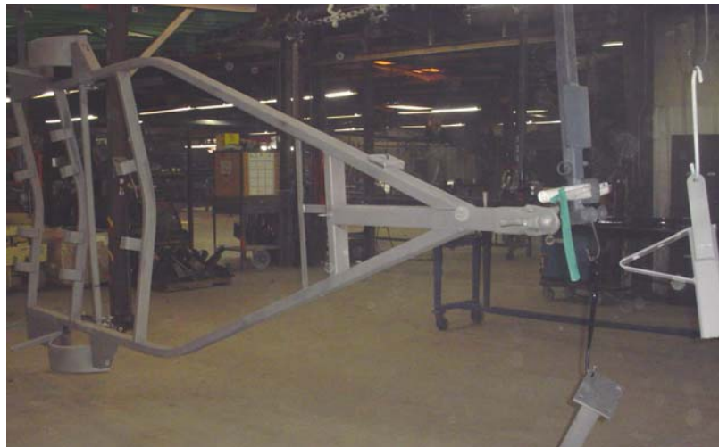
Trailer hanging on monorail, before going into prime booth
