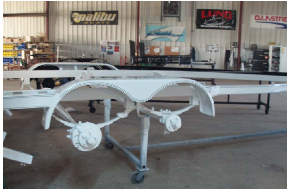
Painted trailers are assembled (completed) in the Finish Line
